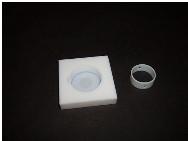
Fig. 1. PTFE cavity for containment of the acetone — shown on the left hand side of the picture, and perforated PTFE ring used as a support of the polymer disc — shown on the right hand side of the picture.
